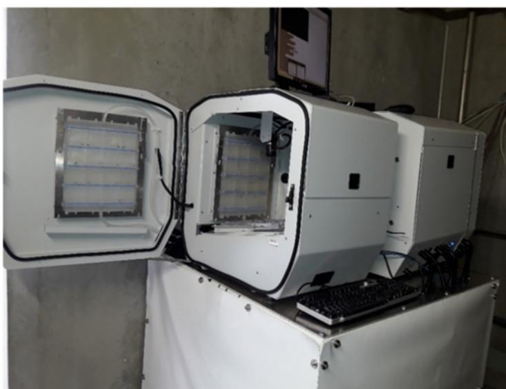
**Figure 3: Station de biosurveillance ToxMate®**
